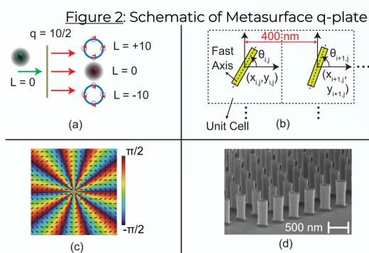
Metasurface devices have the unique capability to structure light in both polarization and phase at a sub-wavelength scale (see Fig. 2(b)). Furthermore, LC devices are often prone to damage under high intensity illumination that is required to perform nonlinear optical measurements.
